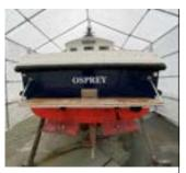
1. Osprey in the tent ready for the cutting and fabrication of a new transom door to facilitate easier access to the boat from her tender as she is kept on a river mooring.
