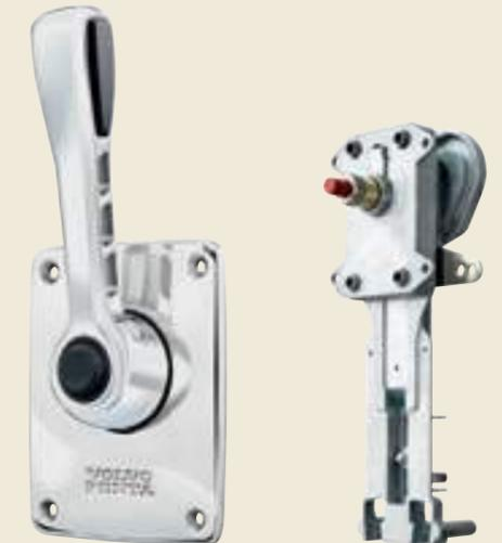
The sailboat control was developed with easy upgrading from older installations as a priority. This means that the control lever can be mounted directly onto an existing Volvo Penta control mechanism. Different combinations of control lever, mechanism and cover can be used, depending on whether it's a new installation, upgrade from a 100x121 mm cover plate or upgrade from a 107x166 mm cover plate.
