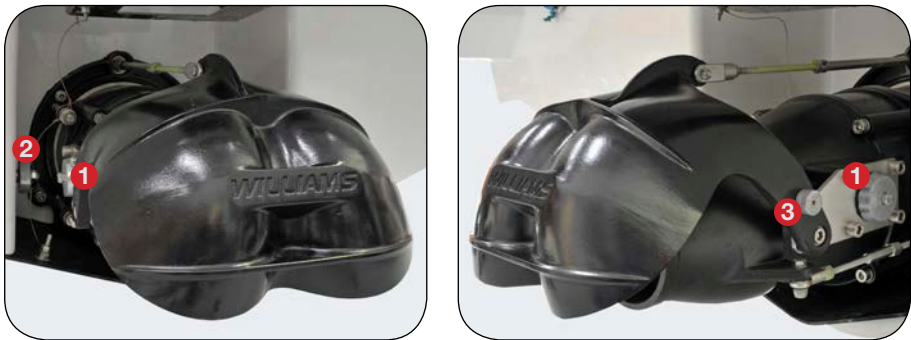
1 Pump anodes 2 Hull anode 3 Reverse bucket anode
